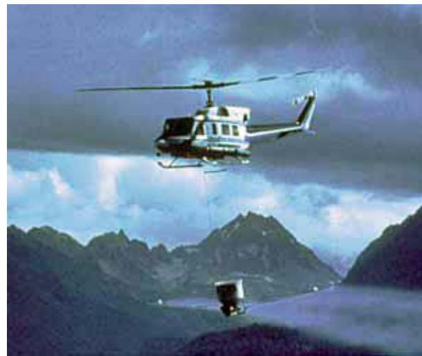
Figure 4. Helicopter with Dispersant Spray Bucket
