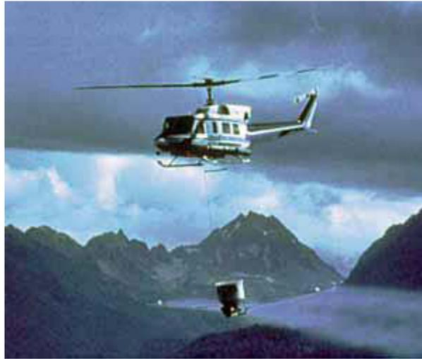
Figure 4. Helicopter with Dispersant Spray Bucket
